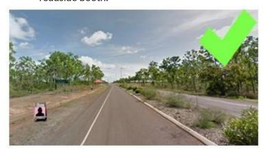
On un-divided road, single sign up to 1.5m<sup>2</sup> in area, on each approach, between 100m to 200m in advance of the mobile roadside booth. 1
