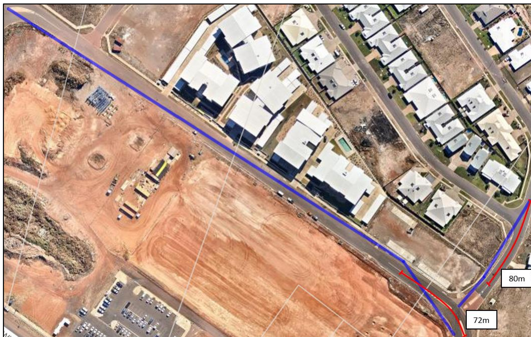
Figure 5.1: Available Stopping Sight Distance
